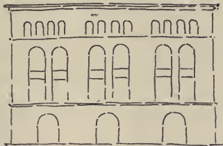
153. Variation of openings with continuous piers.
