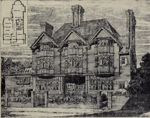
70. Residence, Frank Hall, Hampstead, London. R. Norman Shaw, Architect. An example of three equal subordinate gables.
