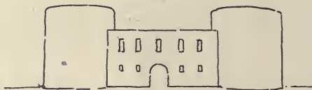
132. Uneven number of openings in central link.
