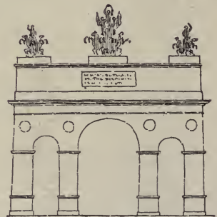
237. The niches in the piers are here increased until they count as members in a triple group of arches.
