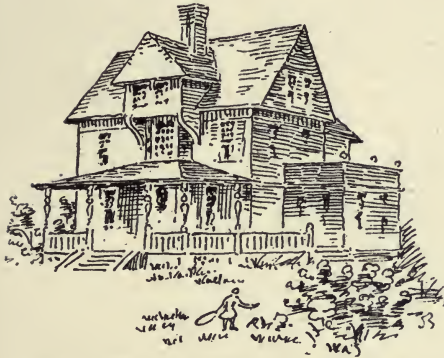
297. The same as 296 with dormer and main roof united by similar treatment.
