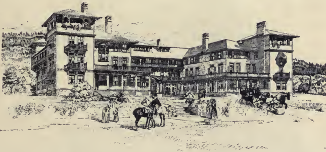
258. Another complex double group. Each member has a tower attached as a subordinate mass.
