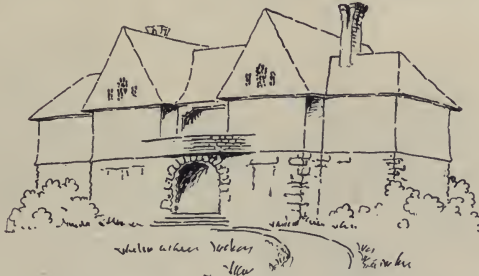
254. Ridge of link not raised. Building extended by appendages, whose ridges are yet lower than that of the link.
