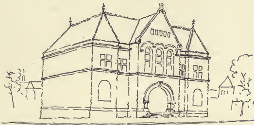
289. An attempt to recompose design of 283. Round tower omitted and replaced by a symmetrical pavilion.
